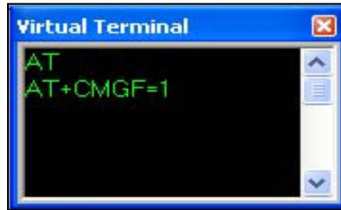
Fig. 7: Virtual Terminal for AT Command of a Receiver
