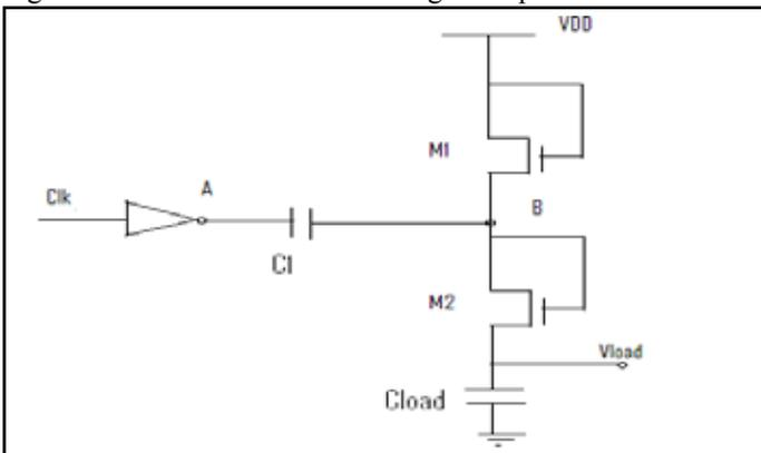
Fig. 2: Basic Single Stage for Charge Pump
