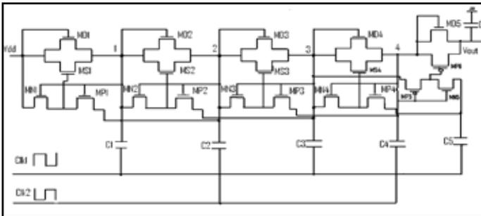
Fig. 1: Low Threshold CMOS Charge Pump
