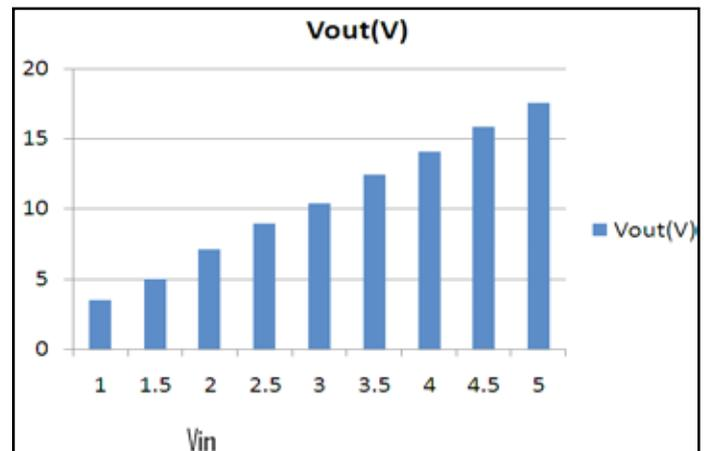
Graph 1 output Voltage vs. Different Input Voltages
