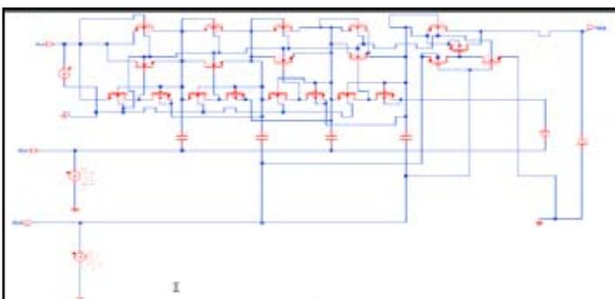
Fig. 3: Schematic of Low Threshold CMOS Charge Pump
