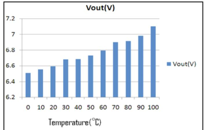
Graph 4 output voltage vs. Different Temperatures
