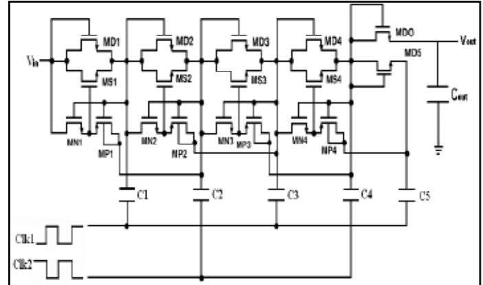
Fig. 8: 4-Stage Dynamic Charge Pump
