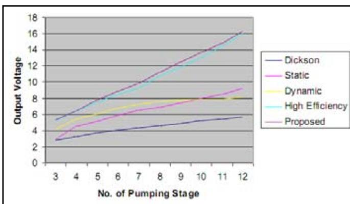
GRAPH 2: Output voltage of Various Charge Pump
