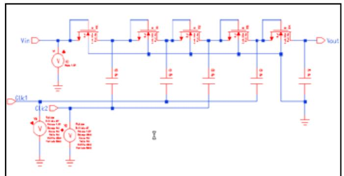
Fig. 3: 4-Stage Schematic of Dickson Charge Pump
