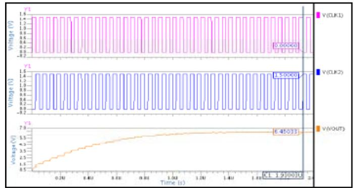
Fig. 13: Output Waveform of 4-Stage Proposed Charge Pump
