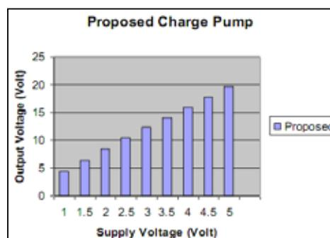
GRAPH 1: Output voltage of Proposed Charge Pump
