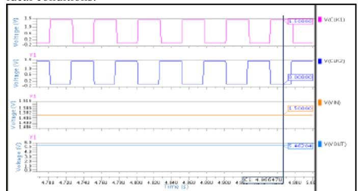
Fig. 10: Output Waveform of 4-Stage Static Charge Pump
