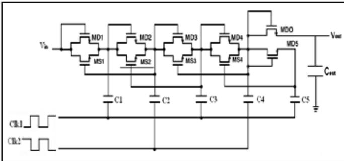
Fig. 5: 4-Stage Static Charge Pump
