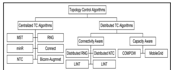
Fig. 3: Algorithms for Topology Control
