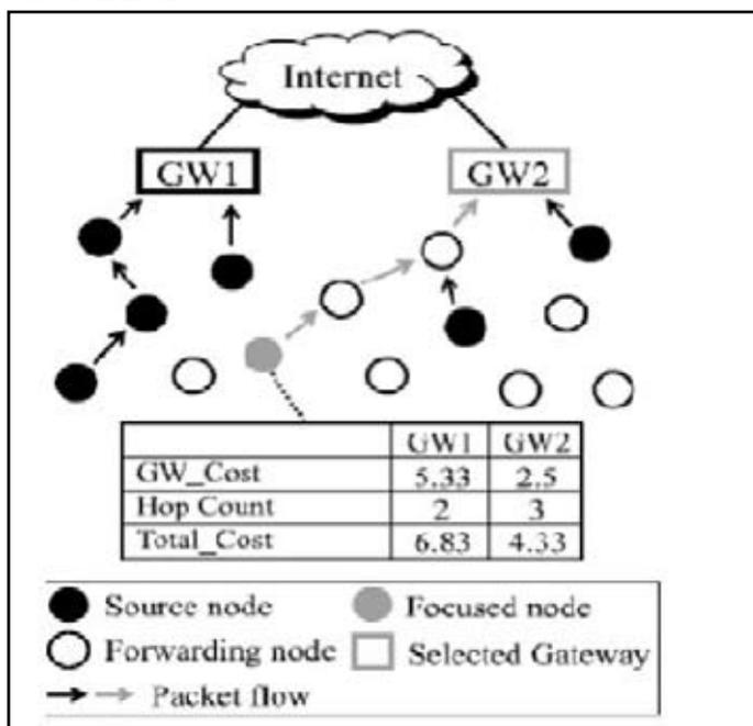
Fig. 2: Load Balancing Gateway
