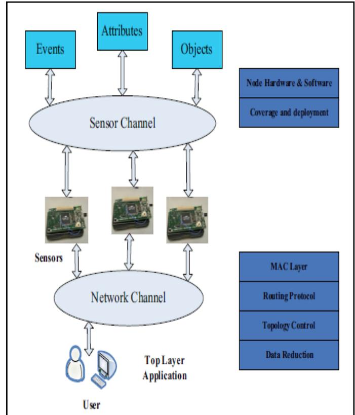
Fig. 1: Wireless Sensor Network Architecture
