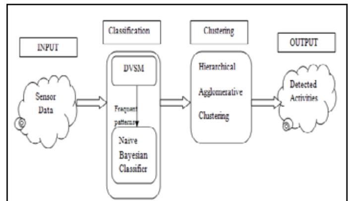
Fig. 3: The Block Diagram of the Activity Recognition System
