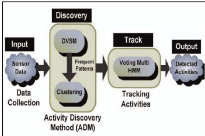
Fig. 2: Main Components of the Existing System for Discovering and Tracking Activities
