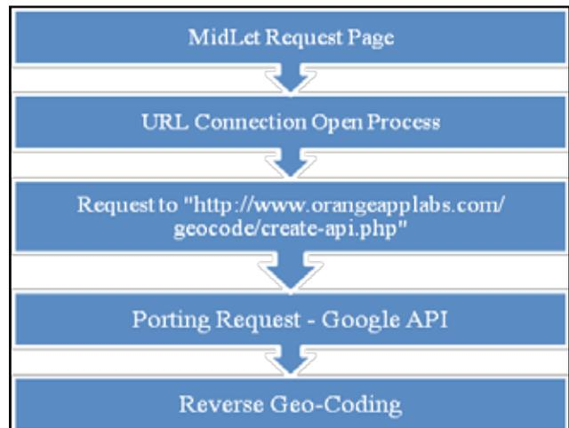
Fig. 3: Request Flow of Geo Location Finding Process
